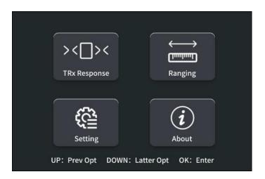
After the Demo board is powered on, the display screen will show the main interface. Users can press the UP/DOWN keys to select different options, and the selected target will be highlighted. Pressing the OK key will enter the corresponding function page.
