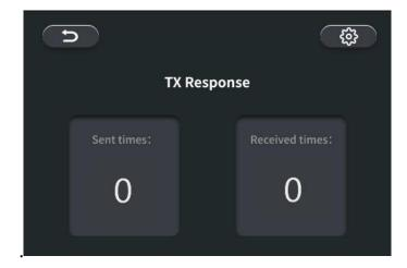
For example, as a transmitter, pressing the OK button to enter this page will start the transmit-receive data test. 'Sent times/Received times' indicates the cumulative number of times data has been successfully transmitted/received, and this value will be displayed in the corresponding box.
