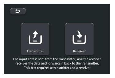
This function requires a transmitter and a receiver to start the test. Press the UP/DOWN key to select the corresponding function, then press the OK key to enter the next page.
